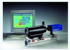
for diffraction limited resolution imaging at high magnification and long working distances Based on high speed, high resolution Cassegrain catadioptic design.
