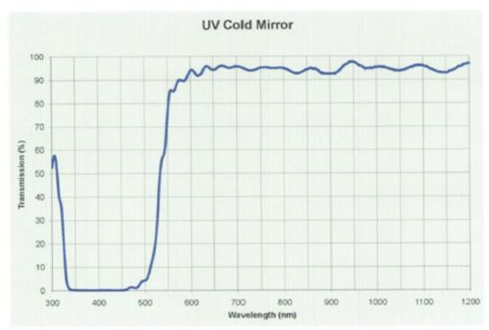
This cold mirror is specially designed to reflect more than 95% average of ultra-violet rays from 350-450nm and transmit more than 90% average 550-1200nm at 45 degrees angle of incidence.
