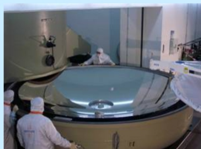
Mirror aluminization in Calar Alto,
