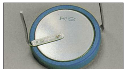
Battery tab welding
