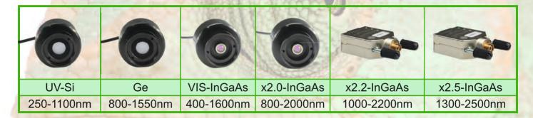
We offer calibrated attenuation filters which extend the range of the free beam heads by up to three orders of magnitude.
