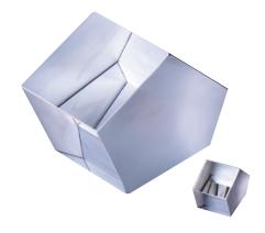
the prism is not possible and also where the path length through an instrument needs to be shortened. Typical applications include range finding, surveying, alignment, and cinephotography. The reflecting faces are coated and the entrance and exit faces have an antireflection coating optimized for 400-700 nm.
