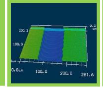
10/10um Min line width /Pitch Any pattern in 600\*600mm +/-5um precision
