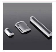
A **Cylindrical lens** is a lens which focuses light into a line instead of a point, as a spherical lens would. It converges or diverges the image in the direction perpendicular to this line, and leaves it unaltered in the direction parallel to its cylinder's axis (in the tangent plane).
