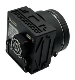
The **EMC-250** is a small, light weight camera with industry standard interfaces. A native connection to the EPIX mf2280 M.2 capture card provides an extremely simple and compact solution for embedded systems. By replacing the standard camera link capture cards and cables with a M.2 card, super high resolution embedded systems and drones are possible. In addition standard camera link is available.
