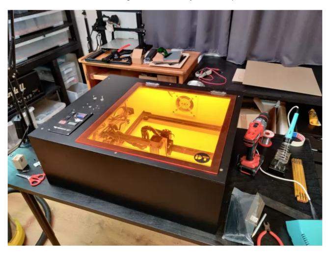
build the enclosure or cover the inside with some thin aluminum sheet or thick foil. This will eliminate any chance of it catching fire, but you should still always be present and watch your laser, as the wood you are engraving on could still catch fire, or there might be some other issue. Once again, you're doing all of this at your own risk.
