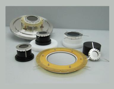
Our Open MCP Detectors consist of one, two or three MCP (micro-channel plate) operating in series.
