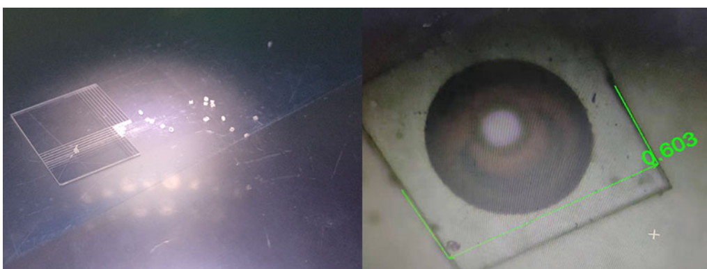
0.6*0.6*0.6mm sapphire cube with wineglass-shape through hole drilling
