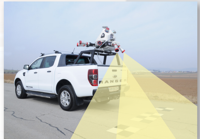
VMX-2HA equipped with 6 horizontally aligned ball-joint directional RIEGL cameras and two ball-joint mounted pavement cameras with close to NADIR orientation
