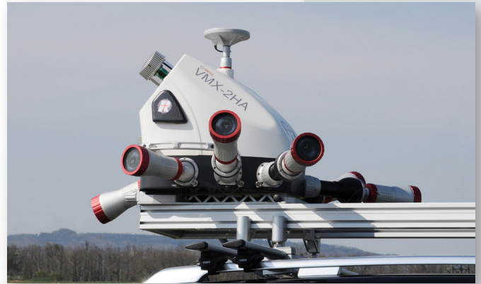
VMX-2HA equipped with 7 ball-joint directional RIEGL cameras
