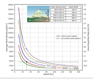
Example: VUX-16023 at 2,400,000 pulses/sec, laser power level 100% altitude 500 ft AGL, speed 30 kn, resulting point density  $\sim$  356 pts/m²
