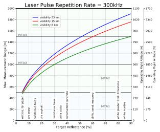
Operating Flight Altitude AGL given for the following conditions: FOV 100°, ambiguity resolved by multiple-time-around (MTA) processing, average ambient brightness, target size ≥ laser footprint, roll angle <±5 deg
