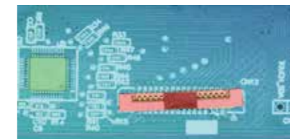
Connector position inspection
